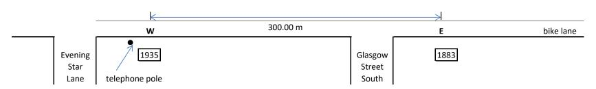
**W** The West nail is located 4.55m east of the centre of the telephone pole at 1935 Sawmill Road, Conestogo. The West nail is located 30cm from the edge of the curb, in the bike lane.
