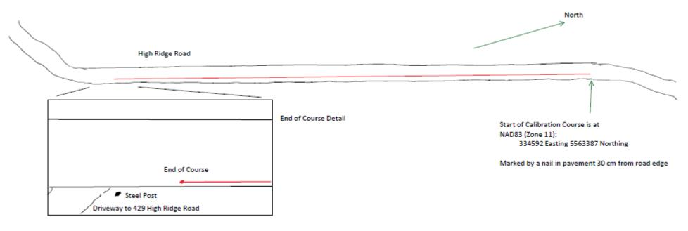
End of course is marked by a nail 30cm from road edge 20.55m measured north of a steel post at the northern edge of the driveway To 429 High Ridge Road.
