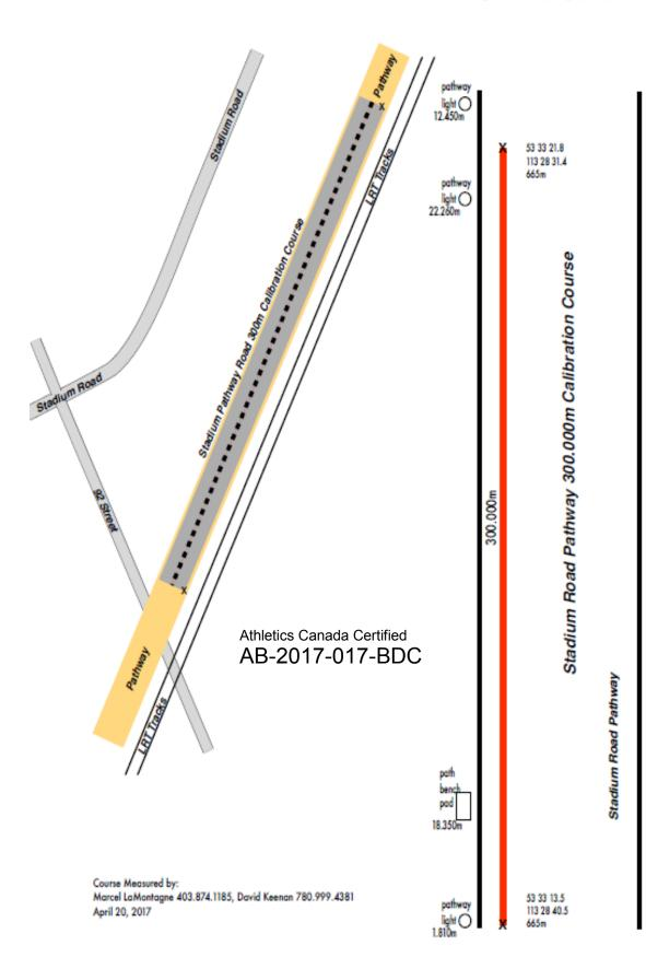
North Reference Measurements (west side, north) pathway light 12.450m (west side, south) pathway light 22.2600m (east side) LRT Slow Sign 12.110m end points located with a mag nail, painted, GPS referenced, photo taken amd measured to 3 permanent objects
