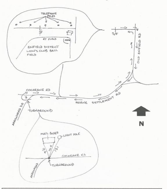
The **turnaround** is in the junction of Cochrane Road and Arrowhead Drive. This is a dirt road so there are no markings. The turnaround can be found by triangulating the point south from the community mailbox pad and the light pole on the north side of Cochrane Road. The point is 9.6 m from the southwest corner of the mailbox pad, 10.4 m from the southeast corner of the pad, and 13.1 m from the light pole.
