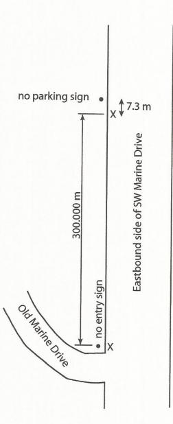
The north pin is located about 15 cm from the edge of the pavement and 7.3 m south of a no parking sign on the eastbound (southwest) side of SW Marine Drive. The pin is at: 49° 14.952' N 123° 14.527' W
