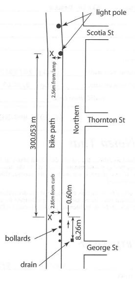
The west pin is located at the 1st light pole east of the intersection of Scotia Street, not counting the light pole at the intersection. The pin is 2.56 m from the centre of the lamp pole.
