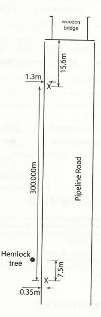
The south pin is located about 15.6m north of the north edge of the wooden bridge on Pipeline road (ie from the edge of the wood). It is 1.3m from the edge of the pavement.
