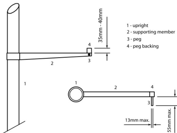
**Figure 8 - Crossbar support** (view from landing area and top view)
