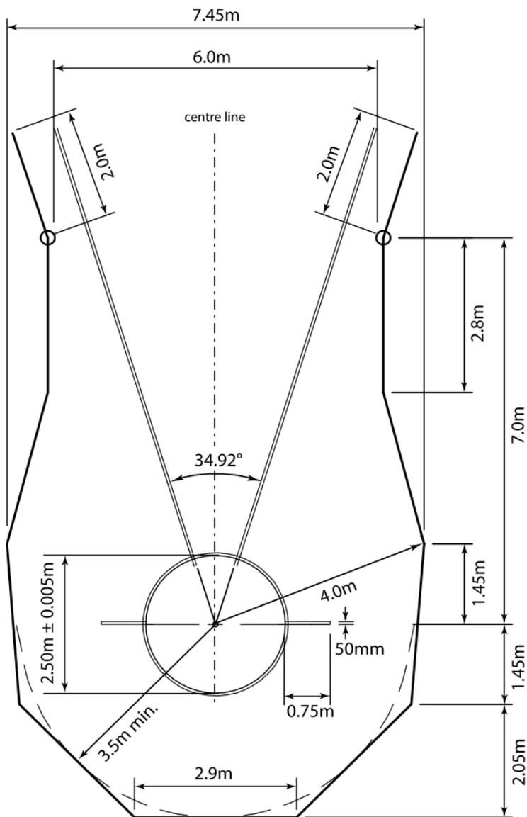
**Figure 23 - Cage for Hammer and Discus Throw with concentric circles
