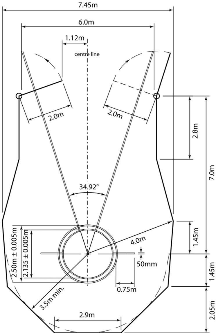
**Figure 22 - Cage for Hammer and Discus Throw with concentric circles
