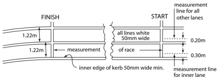
**Figure 1 - Track measurements (infield view)**
