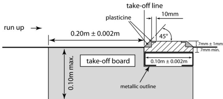
**Figure 10 - Take-off board and plasticine indicator board**
